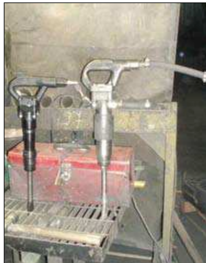
The Grind-All chipping hammer (left) is smaller than a typical 3-in. stroke hammer, but packs the same power.
